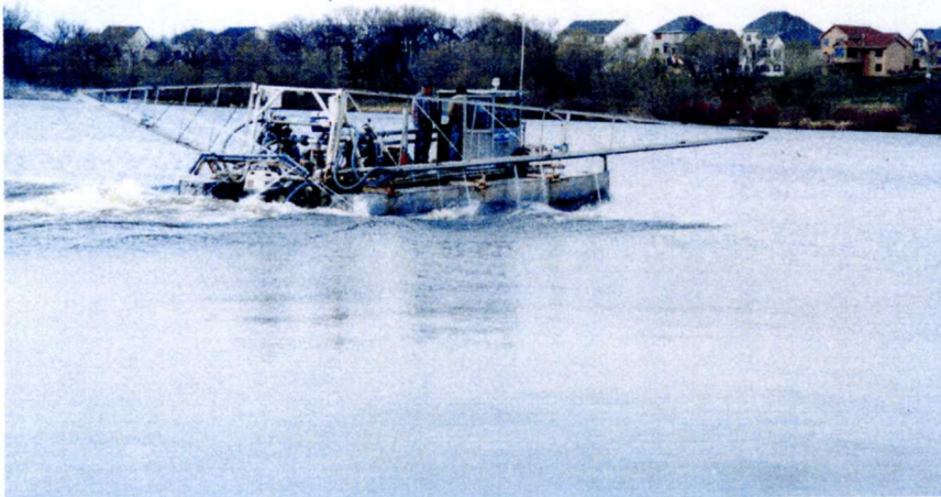
Figure 34. An alum application is generally applied from a barge. This was a lake sediment alum application on Lake Susan in Chanhassen.
